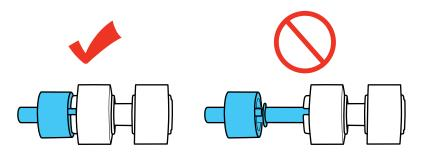
14. Align the notches on the spindle and the scanner, then slide the separation roller into the scanner and gently push it into place. You hear a click when the roller is correctly aligned and locked into place.
